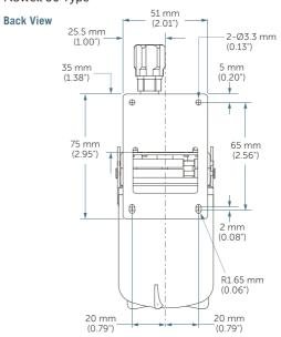
Impact 8G Filter with Impact 2 Manifold - 6.35 mm Super Type Pillar  $^{\odot}$
