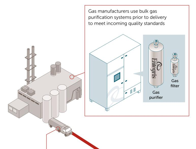
Purified gases can pick up contaminants during storage and transfer
