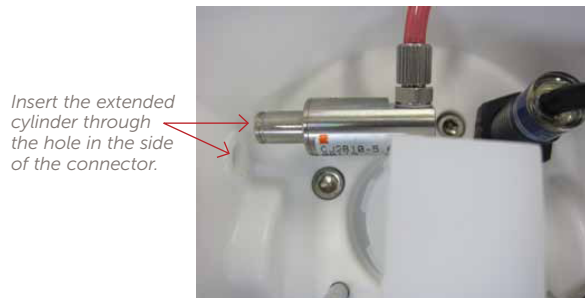
Figure 46. Installing the pneumatic cylinder.
