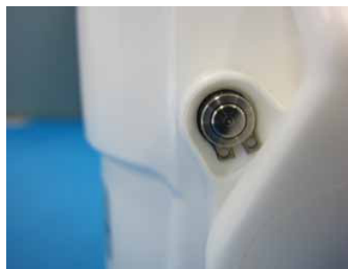
Figure 47. Installed retaining clip.
