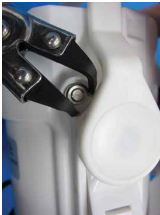
Figure 43. Using the snap ring pliers to remove the retaining clip.
