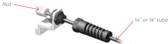
Figure 25. Sliding the nut over the tube.
