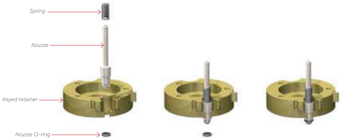
Figure 38. Removing and installing the nozzle, nozzle O-ring and spring.
