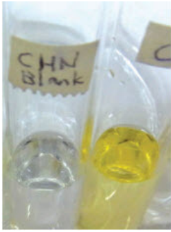
Figure 7. Discoloration of CHN (left: Blank; right: Protego after 1 week soaking).
