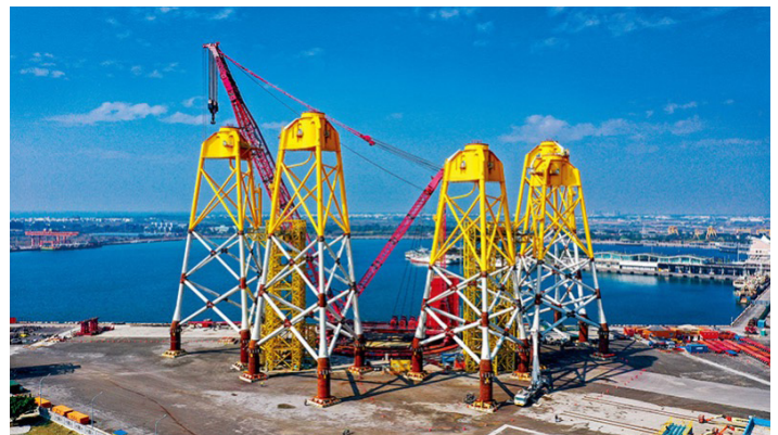
SDMS was invested and founded by China Steel Corporation. It has successfully begun manufacturing of underwater foundations for wind turbines, allowing China Steel to improve its value added by expanding from steelmaking to steel product manufacturing. (Photo Credit: Cheng Szu-Ti) | Expand Photo
