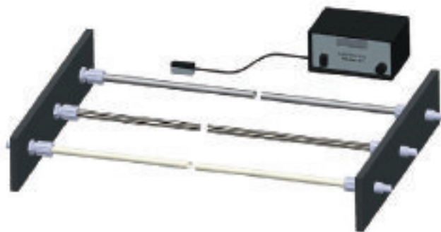
FIGURE 6. Test setup of four-foot and 28-foot tube lengths.
