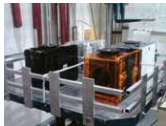
Modified A300 door to match Spectra door closure force
