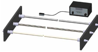
Figure 5: Test setup of four-foot and 28-foot tube lengths
